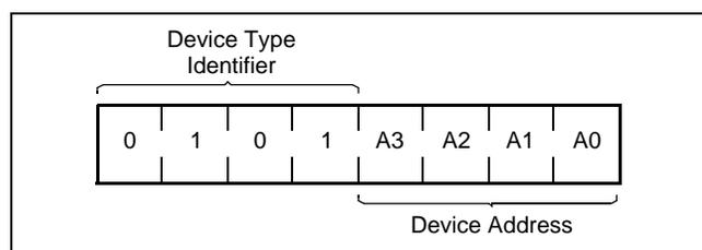
The next four bits of the slave address are the device address. The physical device address is defined by the state of the A0-A3 inputs. The X9221A compares the serial data stream with the address input state; a successful compare of all four address bits is required for the X9221A to respond with an acknowledge.
