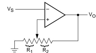
$$V_{UL} = (R_1/(R_1 + R_2)) V_O(\text{max})$$
