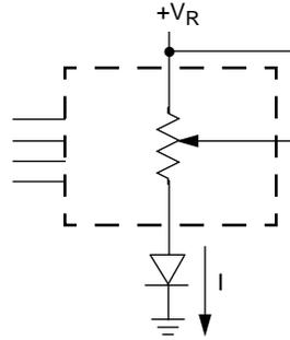
Two terminal Variable Resistor;
