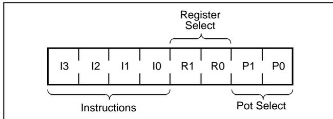
The four high order bits of the instruction byte specify the operation. The next two bits ( $R_1$  and  $R_0$ ) select one of the four registers that is to be acted upon when a register oriented instruction is issued. The last two bits ( $P_1$  and  $P_0$ ) selects which one of the four potentiometers is to be affected by the instruction.
