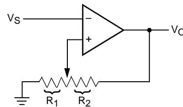
$$V_{UL} = \{R_1/(R_1 + R_2)\} V_O(\text{max})$$
