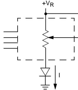
Two terminal Variable Resistor;
