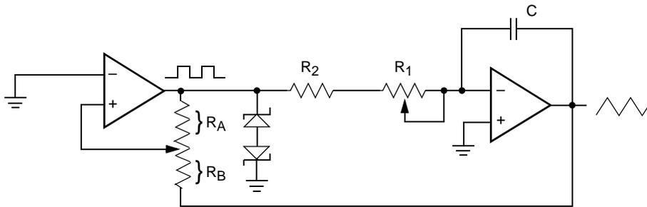
$$\text{frequency} \propto R_1, R_2, C$$
