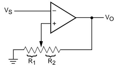
$$V_{UL} = \{R_1/(R_1 + R_2)\} V_O(\text{max})$$
