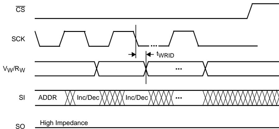
Write Protect and Device Address Pins Timing
