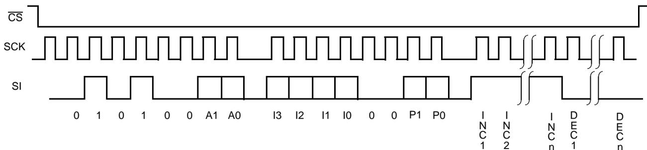
Figure 7. Increment/Decrement Timing Limits
