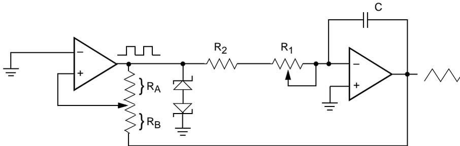
frequency  $\propto R_1, R_2, C$
