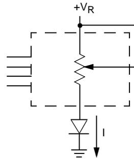
Two terminal Variable Resistor;
