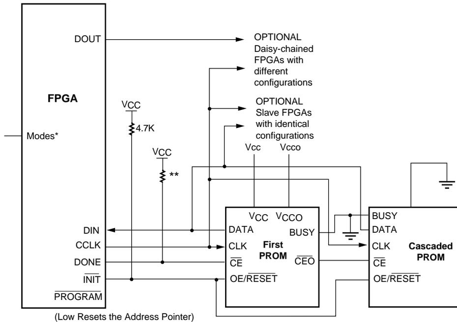
\*For Mode pin connections, refer to the appropriate FPGA data sheet.
