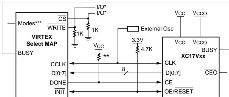
\*CS and WRITE must be pulled down to be used as I/O. One option is shown.
