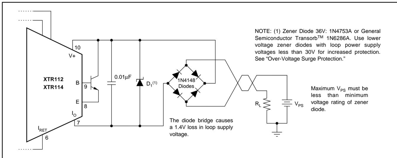
FIGURE 4. Reverse Voltage Operation and Over-Voltage Surge Protection.
