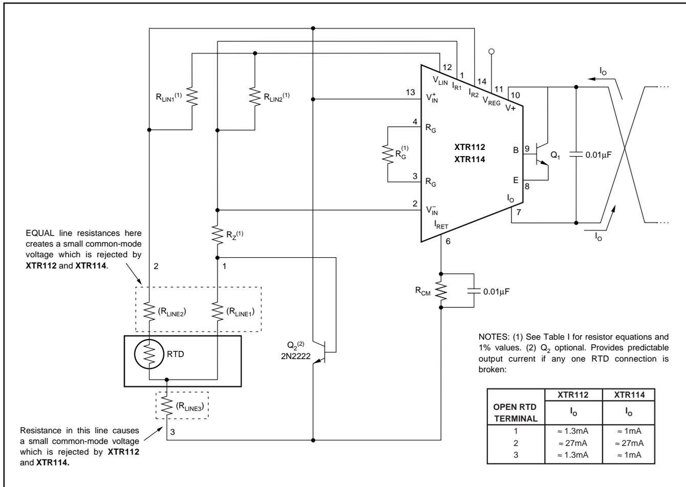
FIGURE 3. Three-Wire Connection for Remotely Located RTDs.
