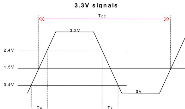
**Figure 9. Single-ended Output Signals (for AC Parameters Measurement)**
