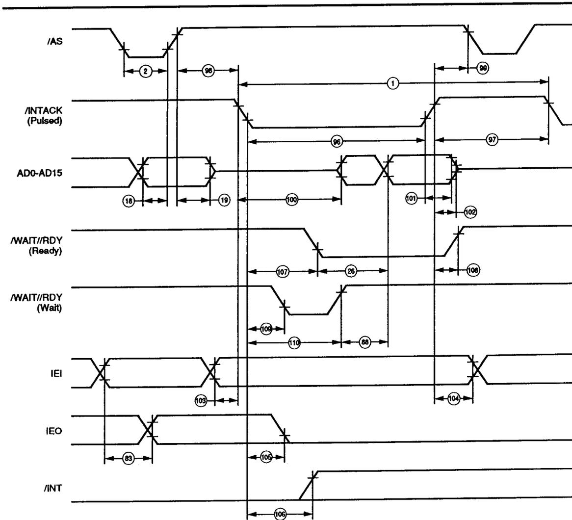
Figure 38. Multiplexed Pulsed INTACK Cycle
