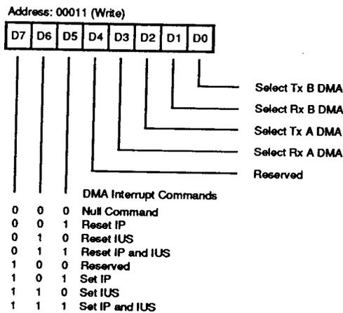
Figure 15. Interrupt Command/Register
