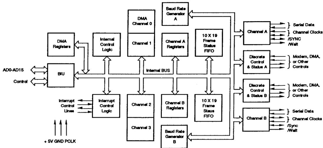
Figure 3. Block Diagram of ISCC Architecture
