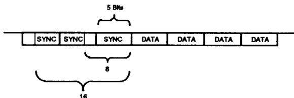
**Figure 5. Detecting 5- or 7-Bit Synchronous Characters**
