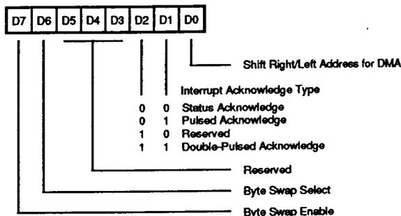
Figure 8. Bus Configuration Register (BCR)
