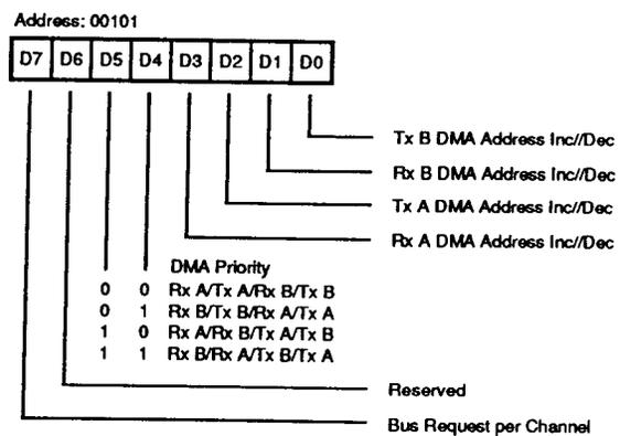
Figure 18. DMA Control Register
