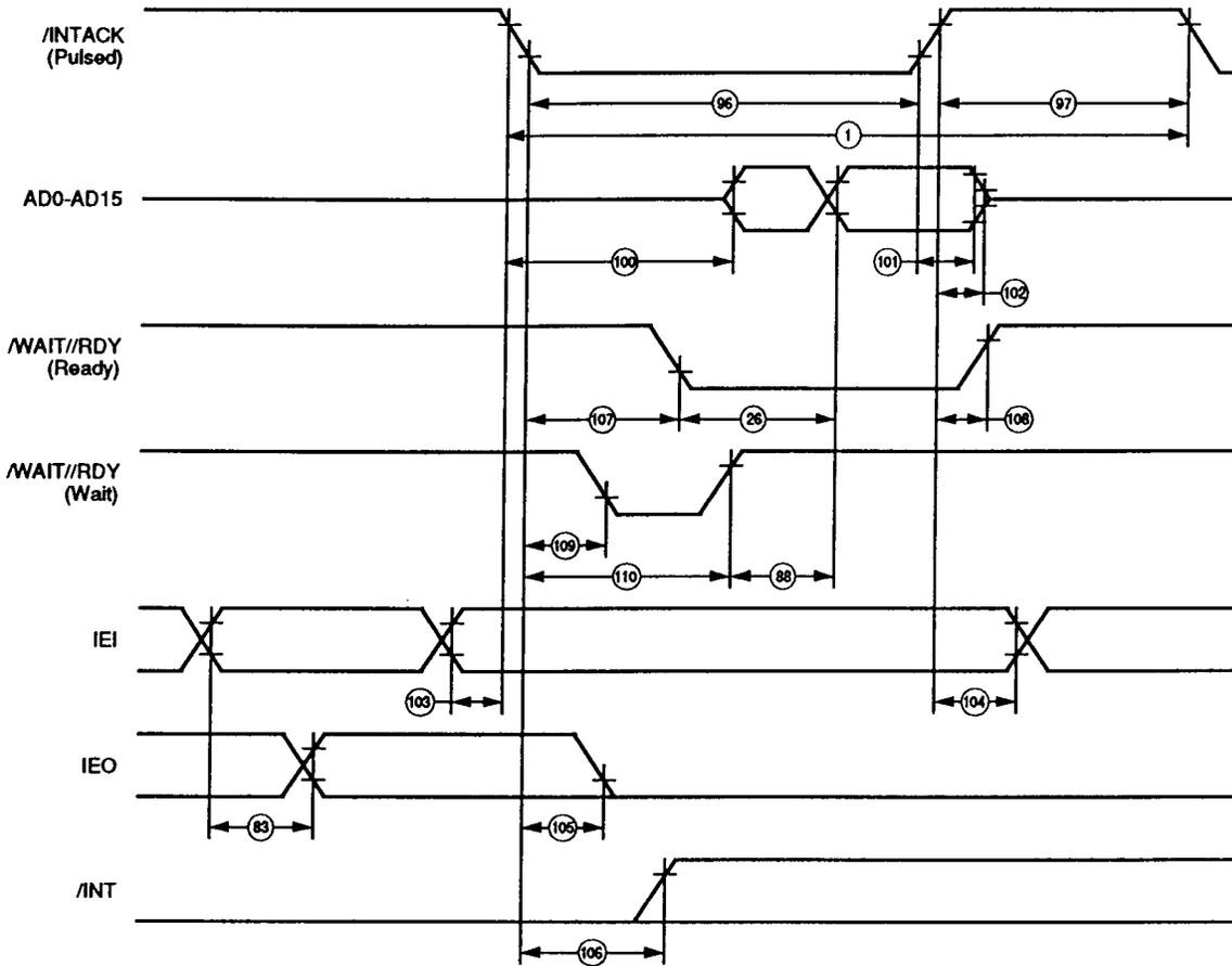
Figure 41. Non-multiplexed Pulsed INTACK Cycle
