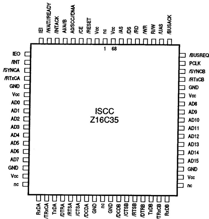
Figure 2. Pin Assignments
