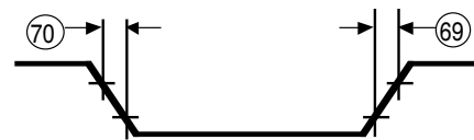
Figure 103. Input Rise and Fall Time (Except EXTAL, /RESET)
