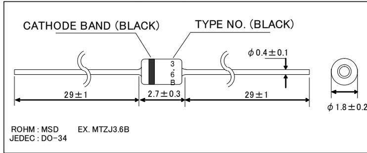
●Taping specification (Unit : mm)
