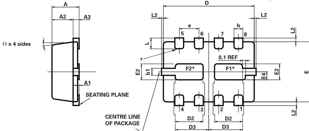
\*Exposed Flags. Solder connection to improve thermal dissipation is optional.
