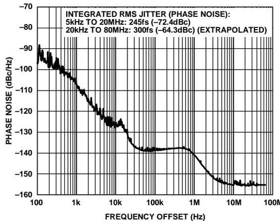
Figure 12. Additive Phase Noise (Output Driver = LVPECL),  $f_R = 19.44$  MHz,  $f_O = 155.52$  MHz, LBW = 1 kHz,  $f_{SYS} = 50$  MHz (Crystal), PLL On with 2x Frequency Multiplier,  $I_{CP} = 375$   $\mu$ A, LF = External (350 kHz)
