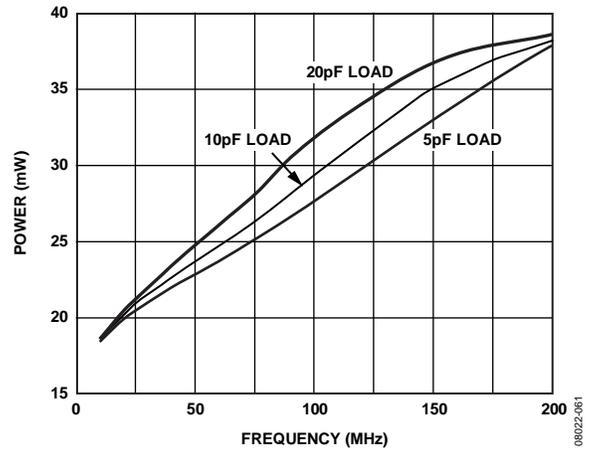
Figure 22. Power Consumption vs. Frequency, 1.8 V CMOS
