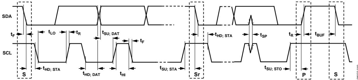
Figure 64. I<sup>2</sup>C Serial Port Timing
