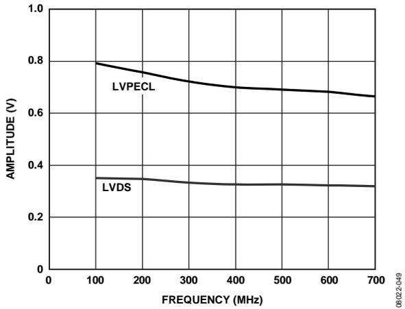
Figure 14. Amplitude vs. Toggle Rate, LVPECL and LVDS
