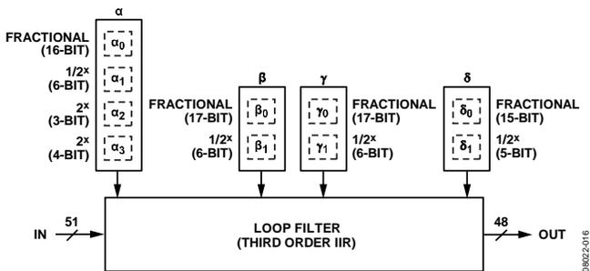
Figure 40. Third Order Digital IIR Loop Filter
