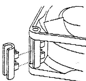
**LZ260/** Spacer of glass-fibre reinforced plastic.
