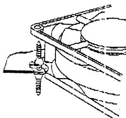
**L2240** The rubber grommet is mounted in the equipment panel with matching hole. The fan rests on the separator piece.
