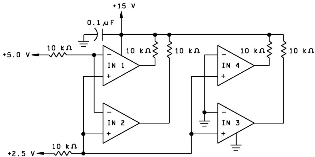
FIGURE 4. Radiation Exposure Circuit.
