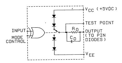
By utilizing an external current limiting structure (accessed via the test point terminal) asymmetrical output currents can be produced from symmetrical power supplies or symmetrical output currents from asymmetrical supplies.
