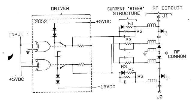
Above is an example using a NEM 2052 driver to actuate a SP2T RF PIN Diode Switch.
