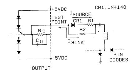
I (SOURCE)  $\cong$  (5-3 (Vf))  $\div$  (R1//R2) I (SINK)  $\cong$  (5-3 (Vf))  $\div$  R2 Vf = DIODE FORWARD DROP
