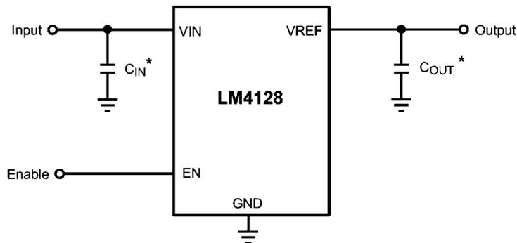
\*Note: The capacitor  $C_{\text{IN}}$  is required and the capacitor  $C_{\text{OUT}}$  is optional.
