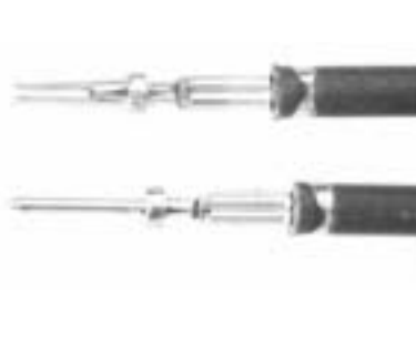
8. Note that there are no unterminated wire strands, and that some strand ends can be seen at the forward edge of the crimp. Also note the insulation is gripped by the smaller secondary crimp. Distortion is at a minimum, both axially and laterally - no sharp edges.
