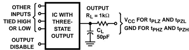
NOTE: Open drain waveforms  $t_{PLZ}$  and  $t_{PZL}$  are the same as those for three-state shown on the left. The test circuit is Output  $R_L = 1k\Omega$  to  $V_{CC}$ ,  $C_L = 50pF$ .
