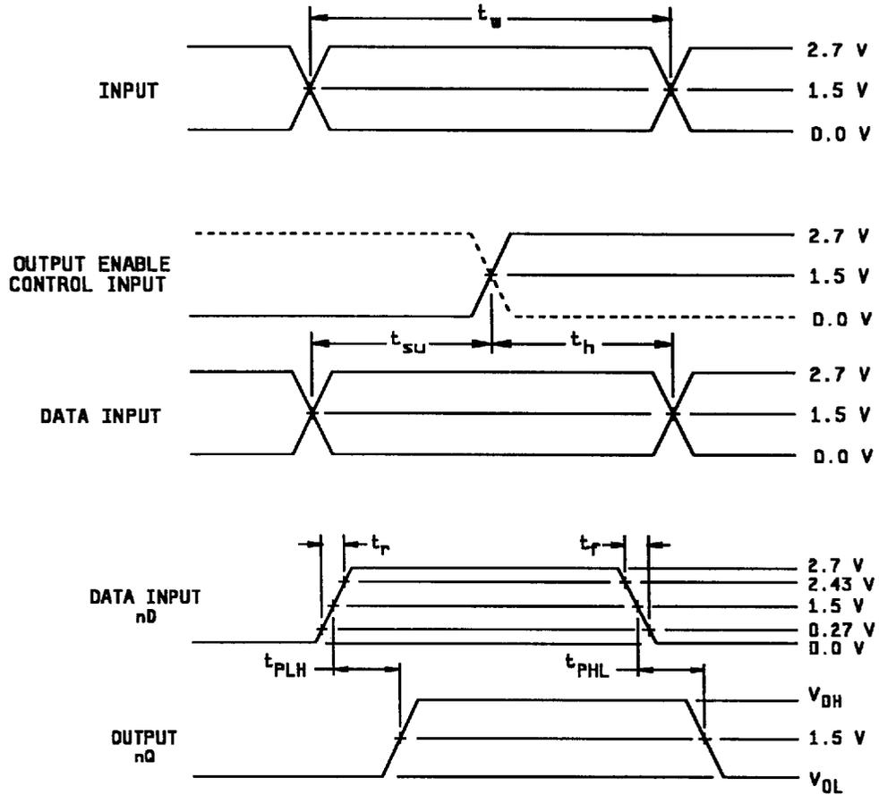
FIGURE 5. Switching waveforms and test circuit.
