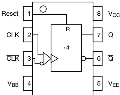
Figure 1. Logic Diagram and Pinout Assignment
