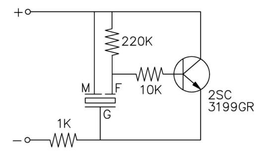
The current consumption and the sound pressure level are measured by using the recommended driving circuit shown above.
