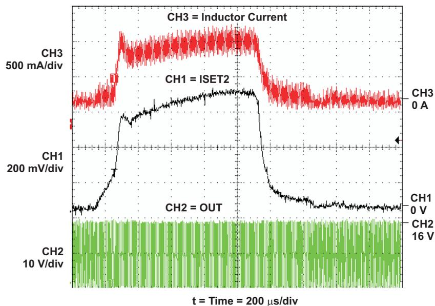
Figure 16. Current Sense Amplifier Charge Current Waveform
