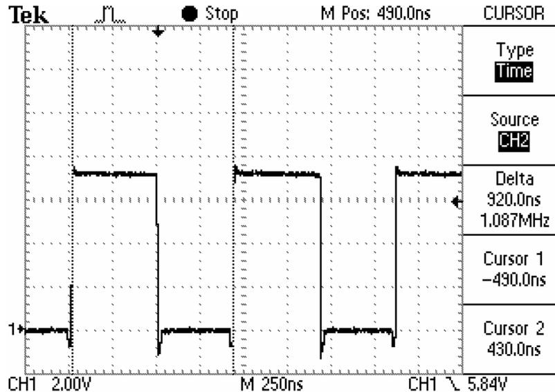
Fast Charge: This is captured during the constant-current phase. The two negative spikes are the result of the short delay when switching between the top and bottom FETs. The break-before-make action prevents current shoot-through and results in a body diode drop below ground potential during the *break* time.
