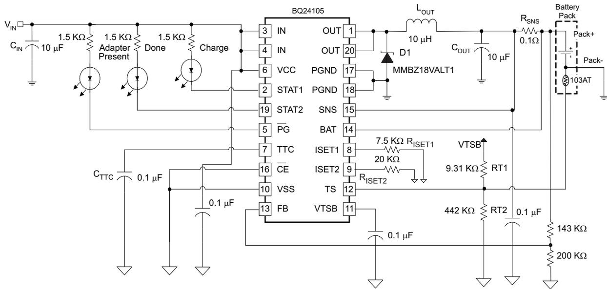
Figure 19. 1-Cell LiFePO<sub>4</sub> Application
