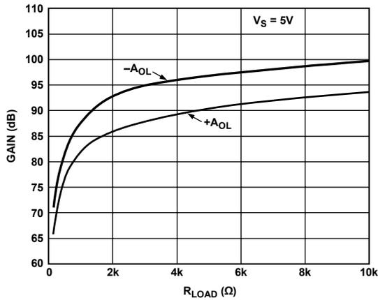
Figure 20. Open-Loop Gain ( $A_{OL}$ ) vs.  $R_{LOAD}$
