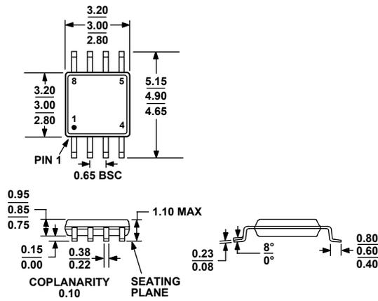
Figure 57. 8-Lead Mini Small Outline Package [MSOP] (RM-8)
