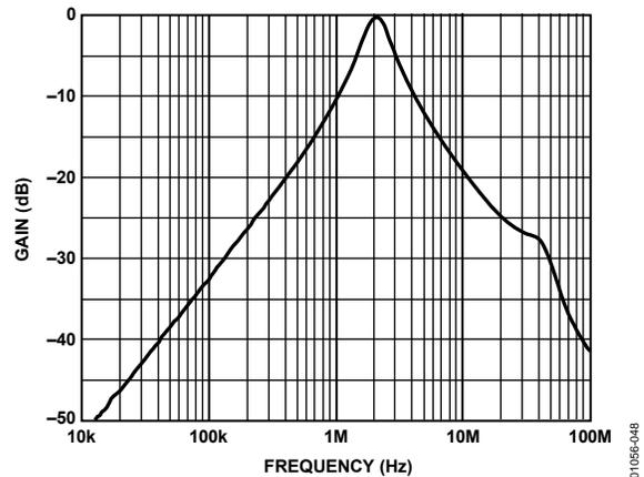
Figure 48. Frequency Response of 2 MHz Band-Pass Filter
