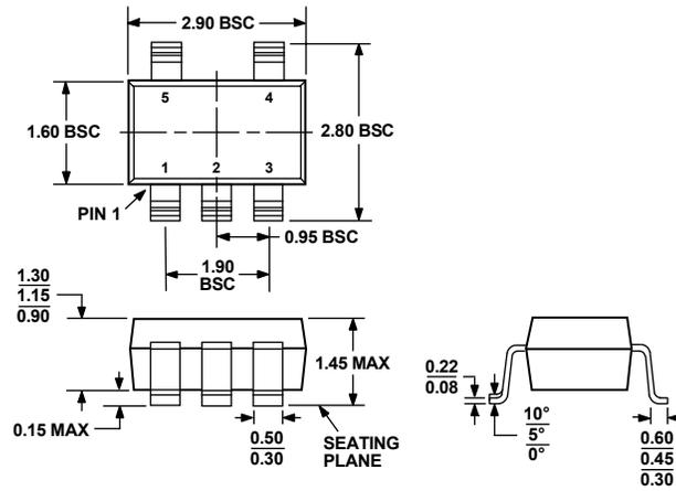
Figure 56. 5-Lead Small Outline Transistor Package [SOT-23] (RJ-5)
