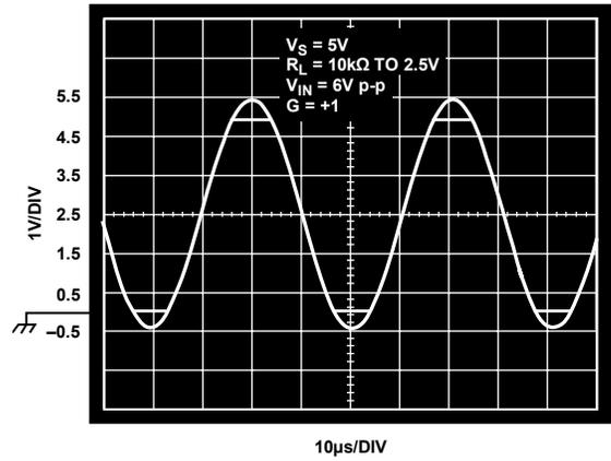
Figure 36. Output Voltage
