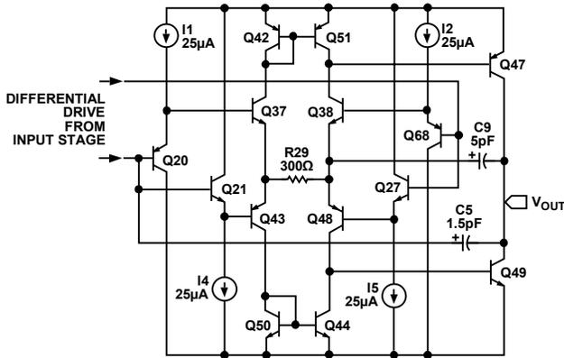
Figure 44. Output Stage Simplified Schematic
