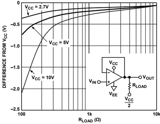
Figure 14. +Output Saturation Voltage vs.  $R_{LOAD}$  @ +85°C
