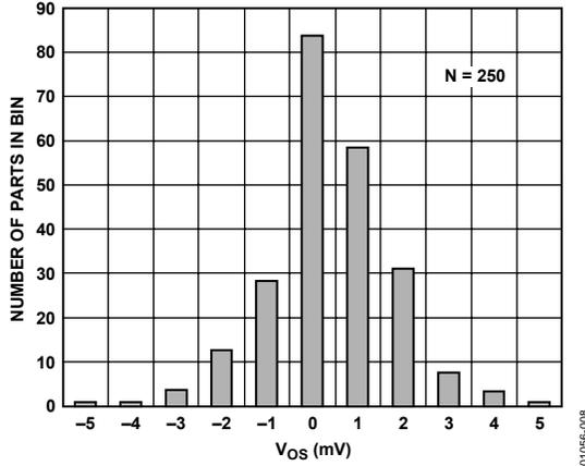
Figure 8. Typical  $V_{OS}$  Distribution @  $V_S = 5V$
