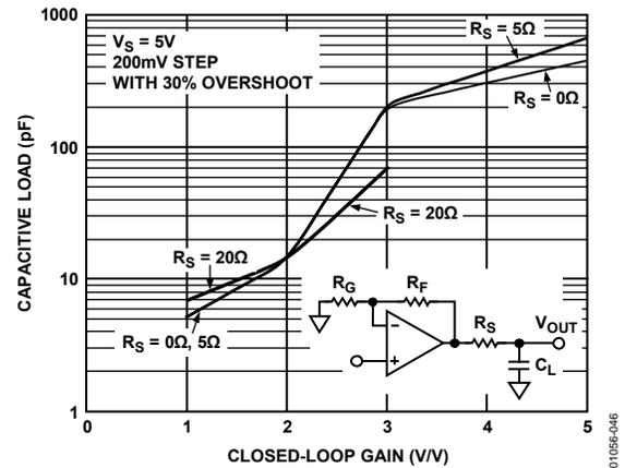
Figure 46. Capacitive Load Drive vs. Closed-Loop Gain
