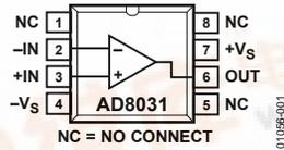
Figure 1. 8-Lead PDIP (N) and SOIC\_N (R)
