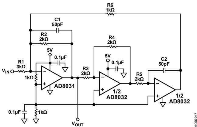
Figure 47. A 2 MHz, Biquad Band-Pass Filter Using AD8031/AD8032
