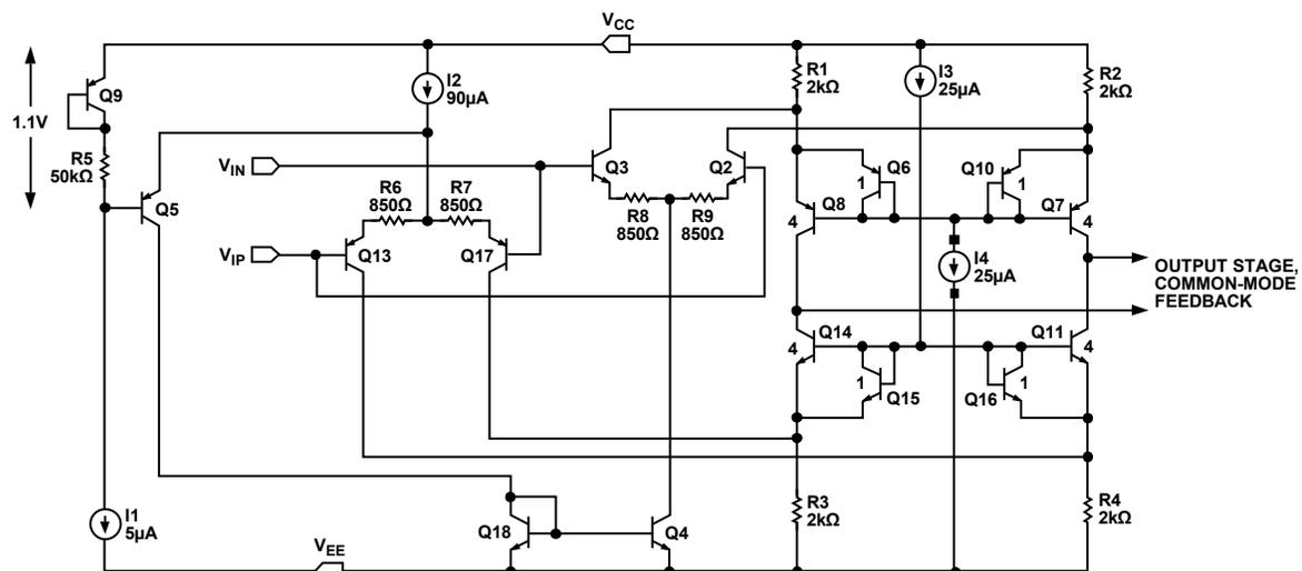
Figure 43. Simplified Schematic of AD8031 Input Stage
