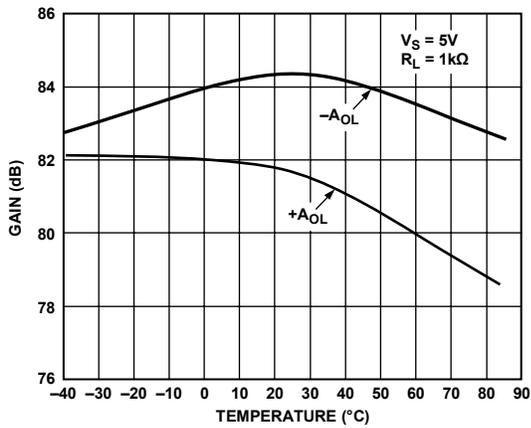
Figure 21. Open Loop Gain vs. ( $A_{OL}$ ) Temperature
