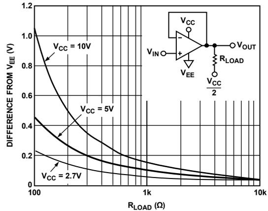
Figure 19. -Output Saturation Voltage vs.  $R_{LOAD}$  @ -40°C
