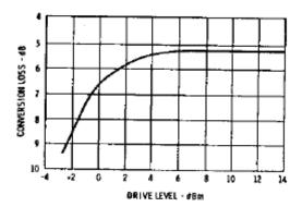
Conversion Loss vs. LO Drive Level: The minimum recommended drive level is +4 dBm. The maximum recommended drive level is +13 dBm.
