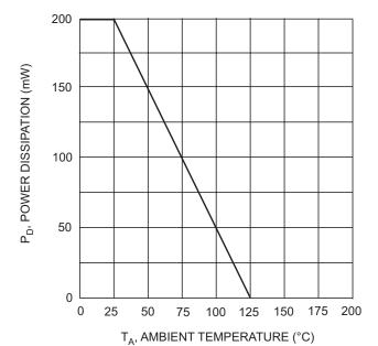
Fig. 1, Max Power Dissipation vs Ambient Temperature
