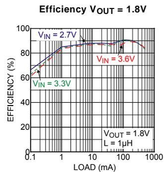
The Figure above shows an efficiency curve. From no load to 100mA, efficiency losses are dominated by quiescent current losses, gate drive and transition losses. By using the Hyper Light Load™ mode the MIC23050 is able to maintain high efficiency at low output currents.
