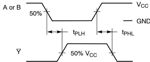
Figure 3. Switching Waveforms
