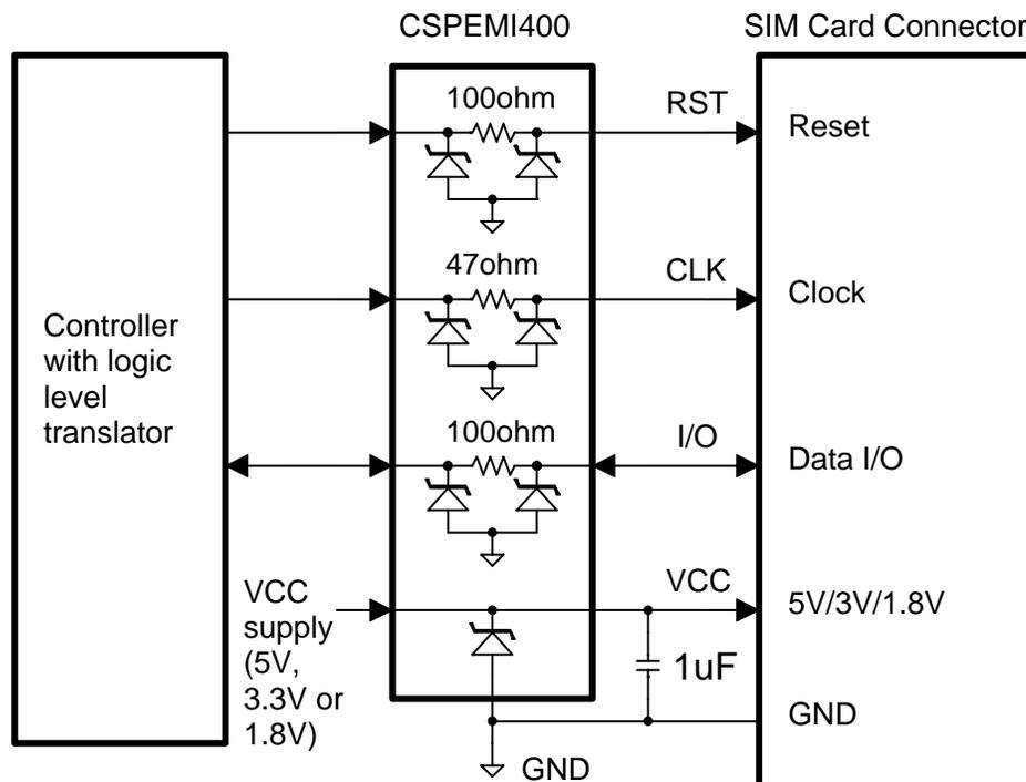
Note: One channel of the CSPEMI400 with a zener diode is not shown on the diagram.
