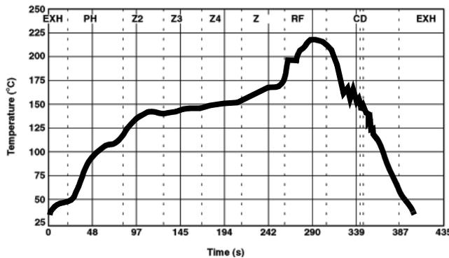
Figure 7. Eutectic (SnPb) Solder Ball Reflow Profile
