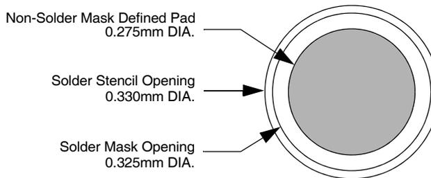
Figure 6. Recommended Non-Solder Mask Defined Pad Illustration
