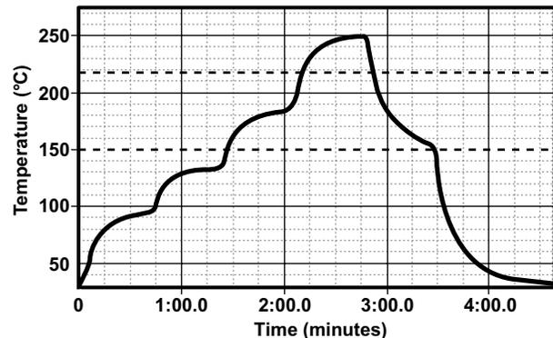
Figure 8. Lead-free (SnAgCu) Solder Ball Reflow Profile
