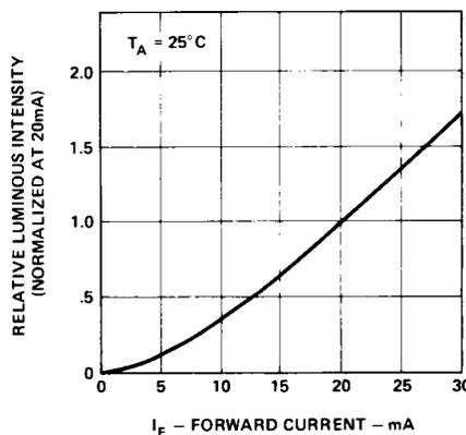
**Figure 18. Relative Luminous Intensity vs. Forward Current.**
