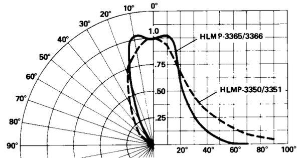
Figure 11. Relative Luminous Intensity vs. Angular Displacement.
