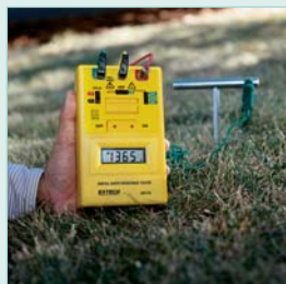
Check resistance between earth and grounding rod.
