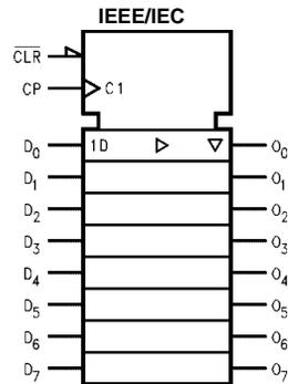
74LVTH273 Low Voltage Octal D-Type Flip-Flop with Clear
