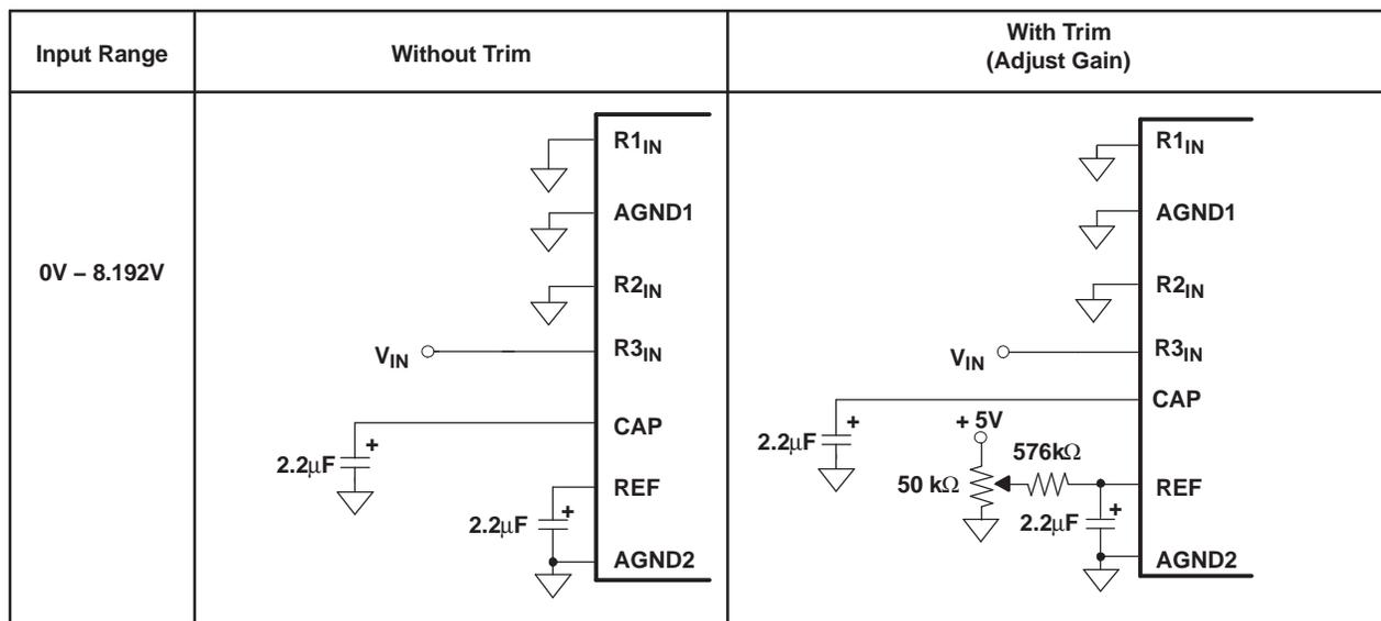
**Figure 29. Offset/Gain Circuits for Unipolar Input Ranges**
