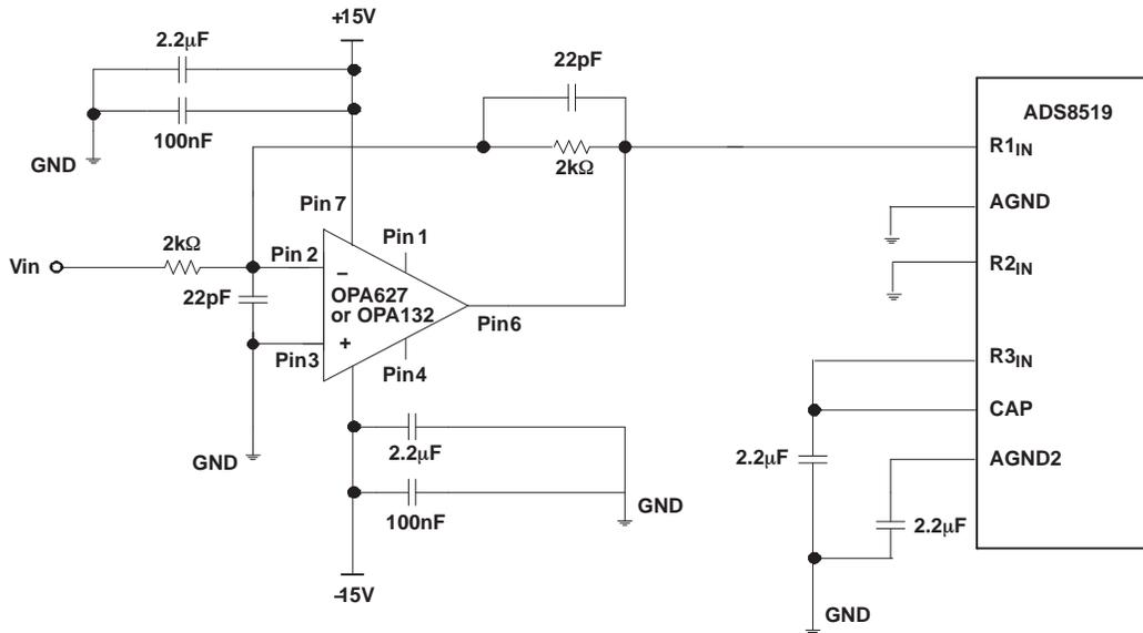
Figure 31. Typical Driving Circuitry (±10V, No Trim)
