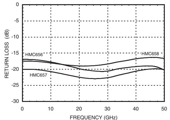
[1] Data taken with die mounted to plate and RF probed through two 1 mil diameter wire bonds.
