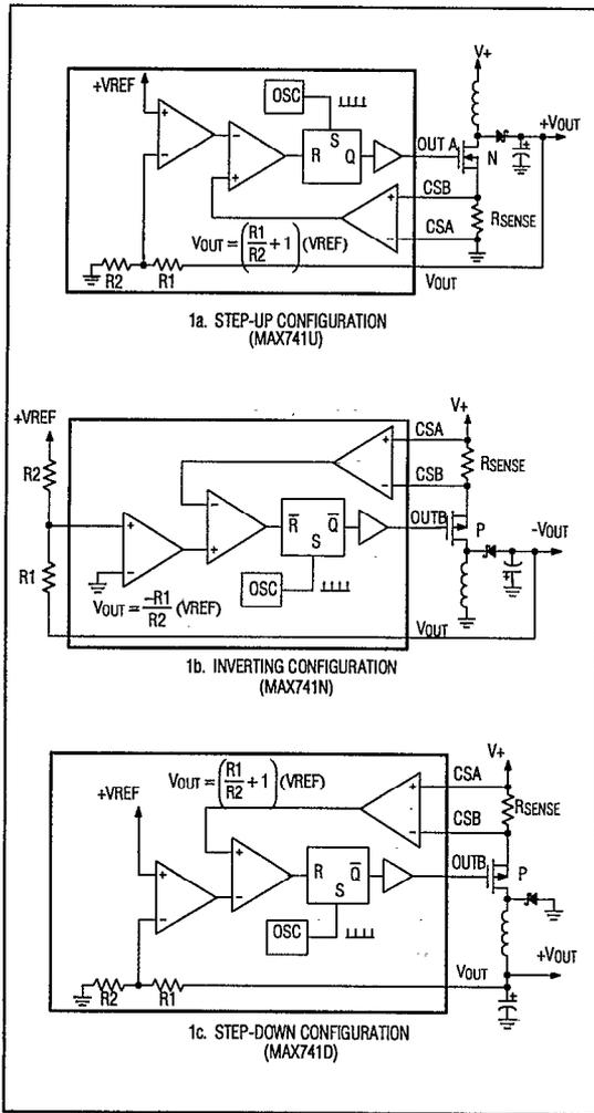
Figure 1. Basic Configurations
