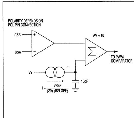
Figure 3. Current Amplifier and Slope Compensation Model
