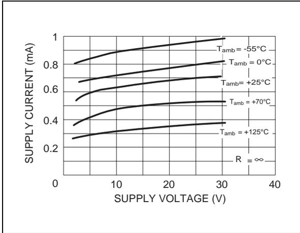
**INPUT CURRENT versus SUPPLY VOLTAGE**
