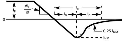
Figure 13.  $t_{rr}$  Waveforms and Definitions
