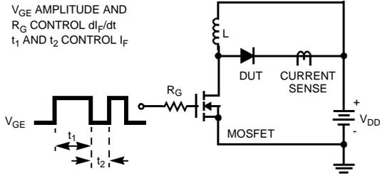
Figure 12.  $t_{rr}$  Test Circuit
