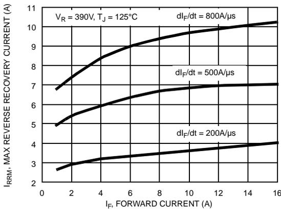
Figure 5. Maximum Reverse Recovery Current vs Forward Current
