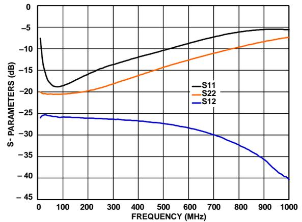
Figure 9. S11, S12 and S22 Vs. Frequency
