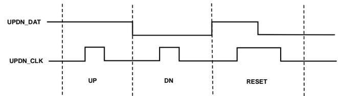
Figure 3. UP/DOWN Timing
