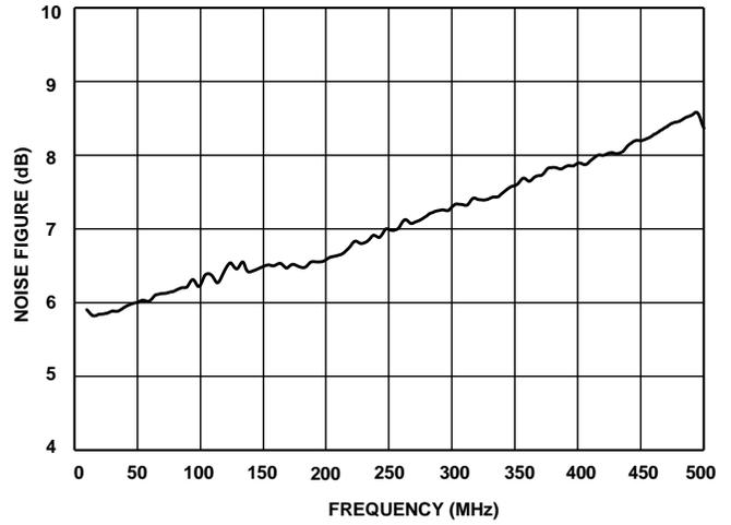
Figure 8. Noise Figure Vs. Frequency at Max Gain
