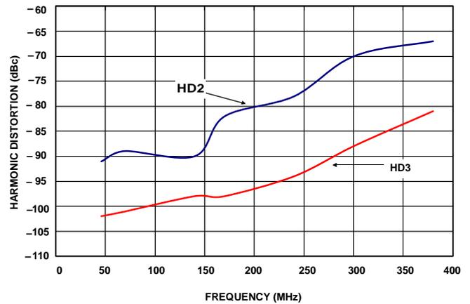
Figure 10. Harmonic Distortion Vs. Frequency 2Vp-p Out
