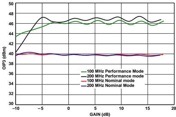
Figure 7. OIP3 Vs. Gain
