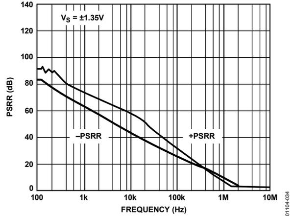
Figure 34. PSRR vs. Frequency at  $\pm 1.35V$
