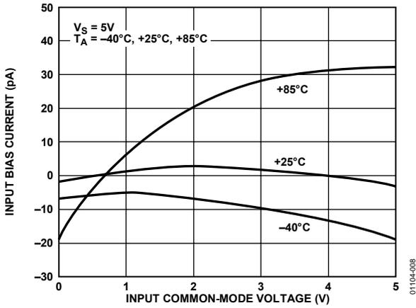
Figure 8. Input Bias Current vs. Input Common-Mode Voltage
