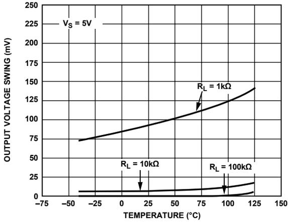
Figure 48. Output Voltage to Supply Rail vs. Temperature
