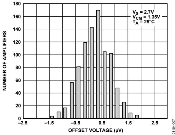
Figure 7. Input Offset Voltage Distribution at 2.7 V
