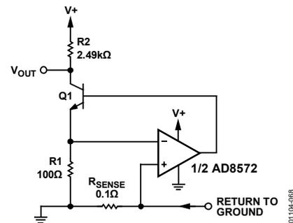
Figure 68. Low-Side Load Current Monitor
