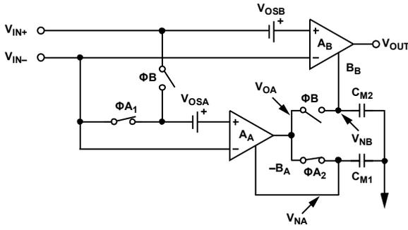
Figure 50. Auto-Zero Phase of the Amplifier
