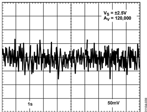
Figure 39. 0.1 Hz to 10 Hz Noise at 5V
