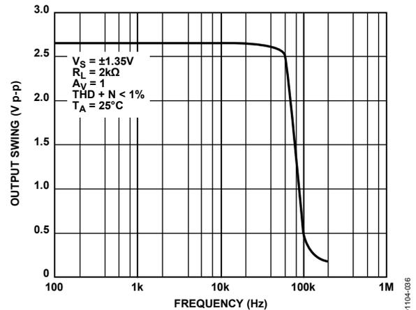
Figure 36. Maximum Output Swing vs. Frequency at 2.7 V
