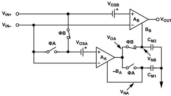
Figure 51. Output Phase of the Amplifier
