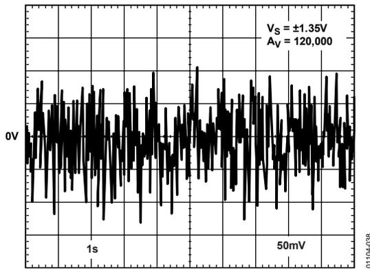
Figure 38. 0.1 Hz to 10 Hz Noise at 2.7V
