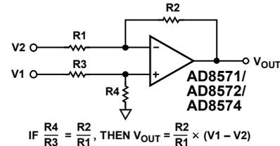
Figure 64. Using the AD857x as a Difference Amplifier
