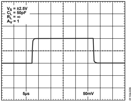
Figure 26. Small Signal Transient Response at 5V
