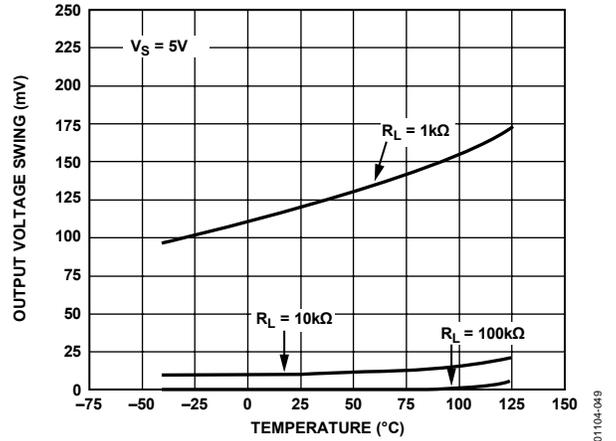
Figure 49. Output Voltage to Supply Rail vs. Temperature
