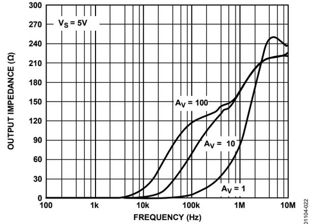
Figure 22. Output Impedance vs. Frequency at 5 V
