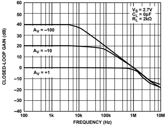
Figure 19. Closed-Loop Gain vs. Frequency at 2.7 V
