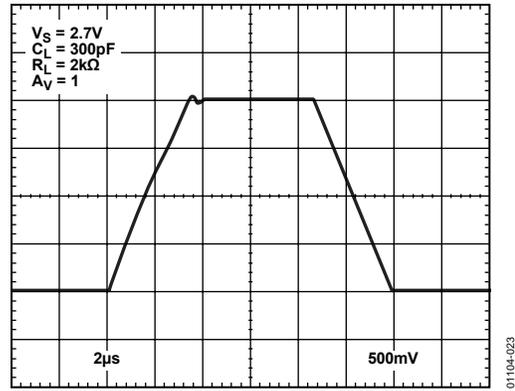
Figure 23. Large Signal Transient Response at 2.7 V
