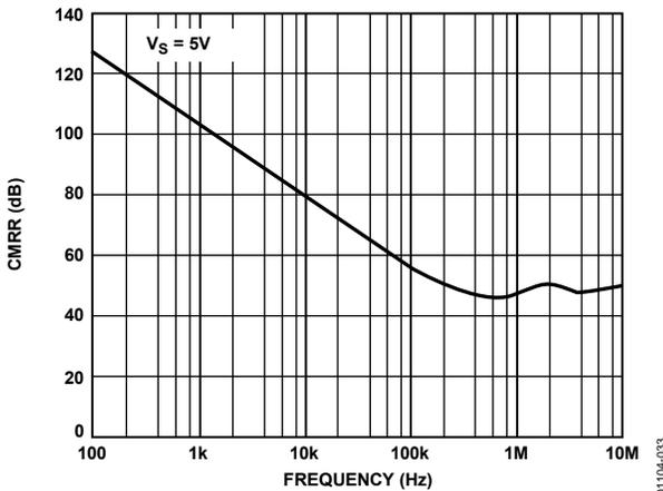
Figure 33. CMRR vs. Frequency at 5 V
