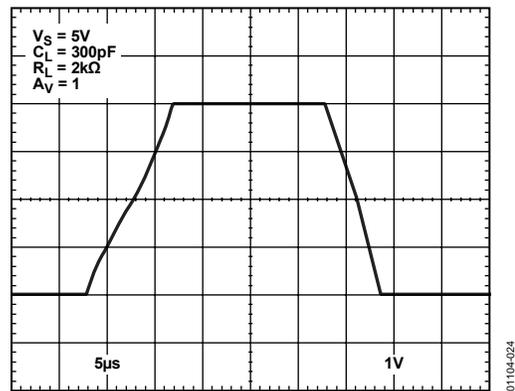
Figure 24. Large Signal Transient Response at 5 V
