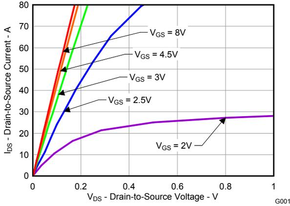
**Figure 2. Saturation Characteristics**
