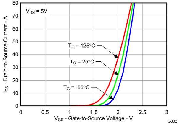
**Figure 3. Transfer Characteristics**
