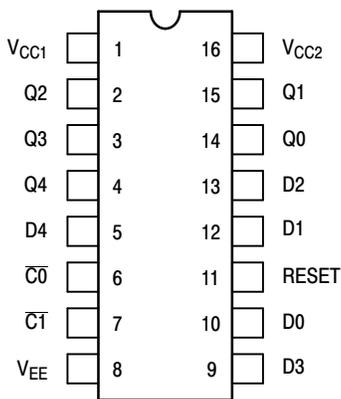
Pin assignment is for Dual-in-Line Package.
