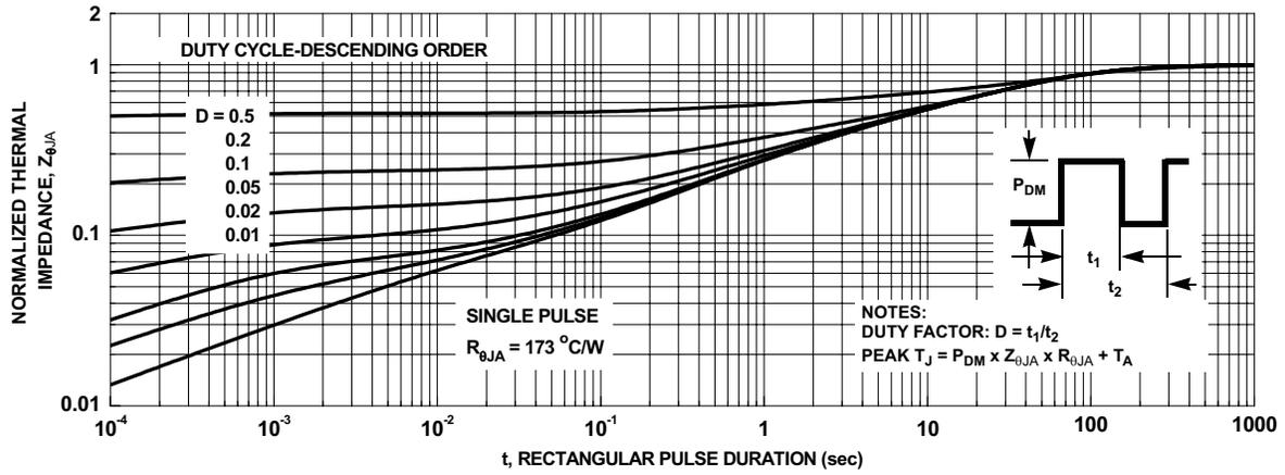
Figure 13. Junction to Ambient Transient Thermal Response Curve
