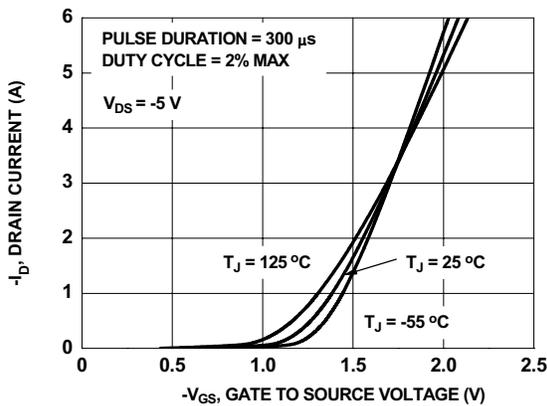
Figure 5. Transfer Characteristics
