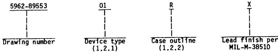
1.2.1 Device type. The device type shall identify the circuit function as follows:
