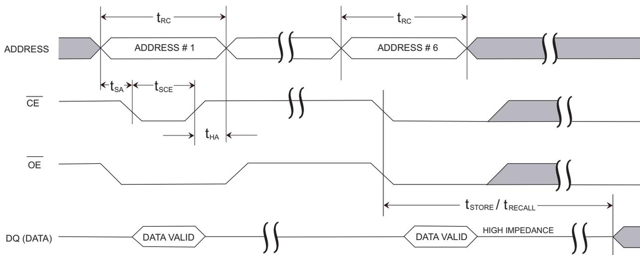
Figure 11.  $\overline{OE}$  Controlled Software STORE/RECALL Cycle [17]
