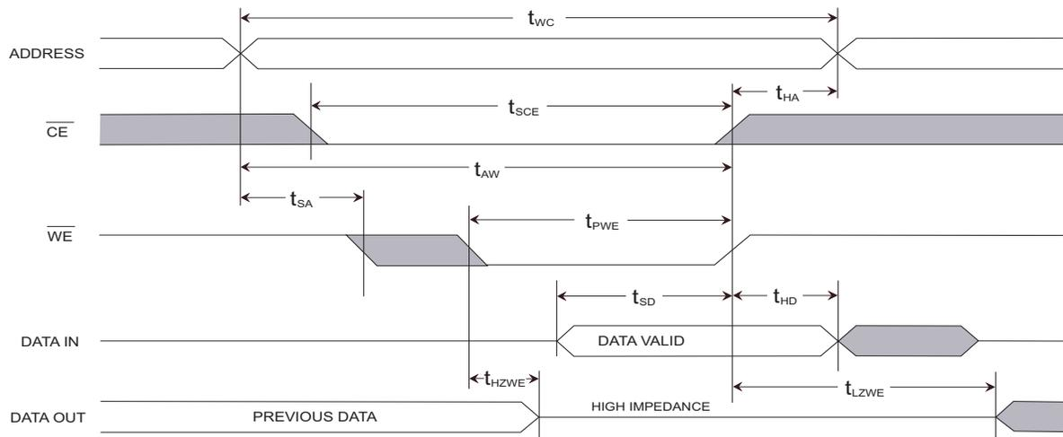
Figure 8. SRAM Write Cycle 2:  $\overline{CE}$  and  $\overline{OE}$  Controlled [11, 12]
