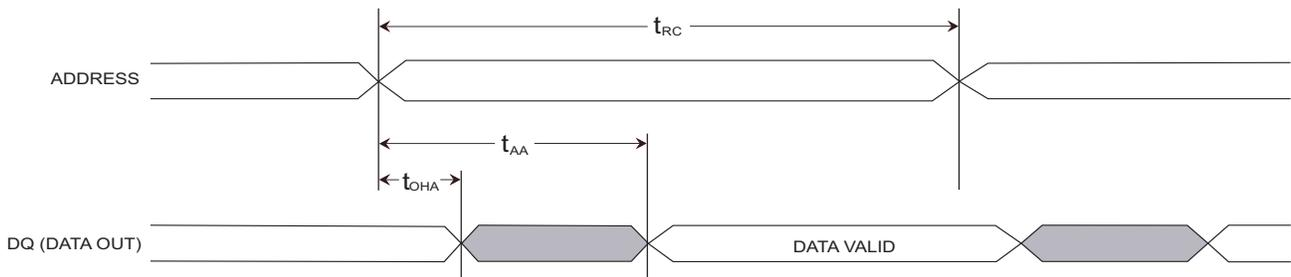
Figure 6. SRAM Read Cycle 2:  $\overline{CE}$  and  $\overline{OE}$  Controlled [7, 10]
