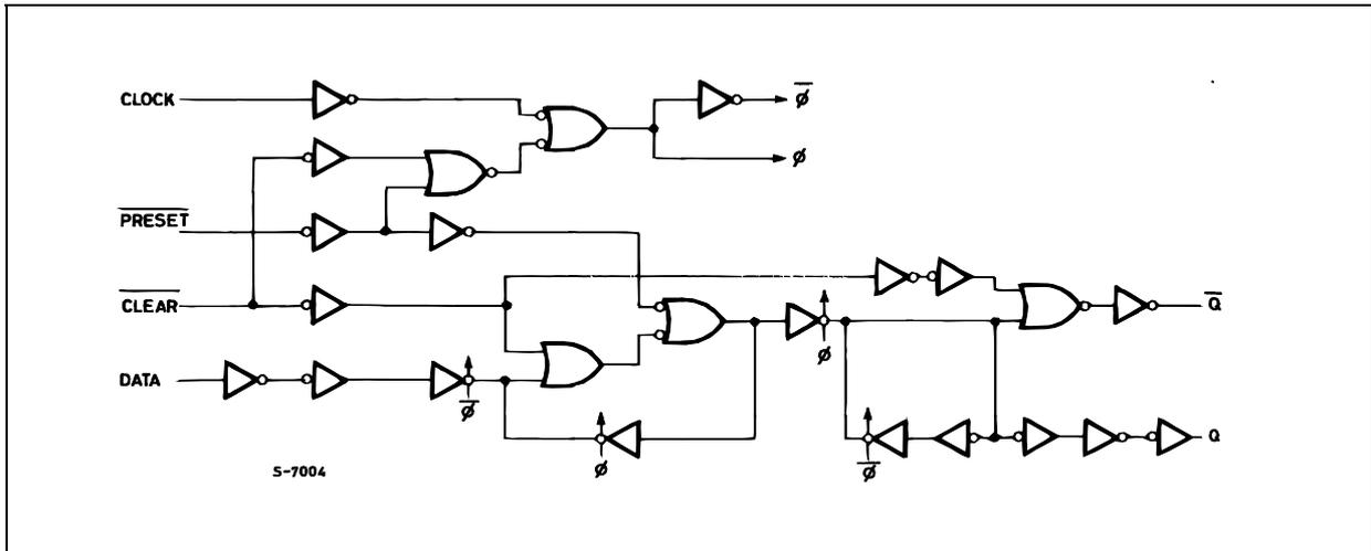
This logic diagram has not be used to estimate propagation delays
