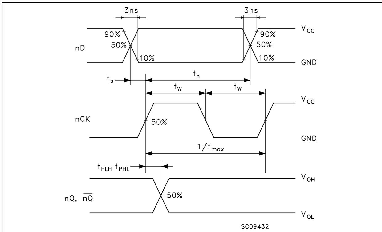
Figure 6: Waveform - Propagation Delays (f=1MHz; 50% duty cycle)
