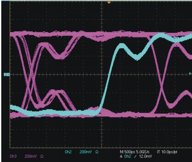
Figure 104. LVDS Eye Diagram - No Internal Termination
