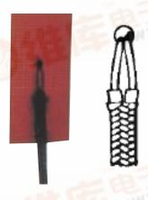
Easily mounted on most surfaces, the 'Stikon™' thermocouple is constructed using 0.25mm diameter wire which is bead welded and embedded in a paper thin laminate intended for surface application by adhesive bonding. These versatile, low cost thermocouples can be used for a wide variety of surface temperature measurements including environmental testing, temperature surveys of electrical components, oven wall temperature, etc. They are designed YWW.DZ for use with standard readout instruments.
