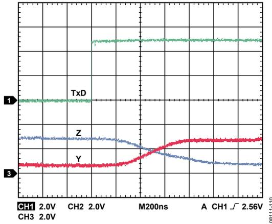
Figure 10. ADM2587E Driver Propagation Delay
