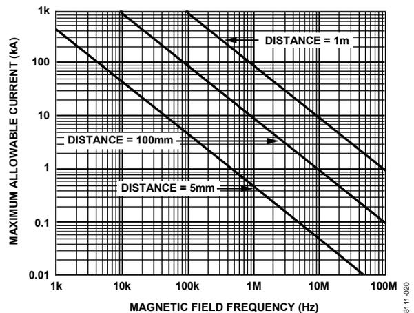
Figure 34. Maximum Allowable Current for Various Current-to-ADM2582E/ADM2587E Spacings
