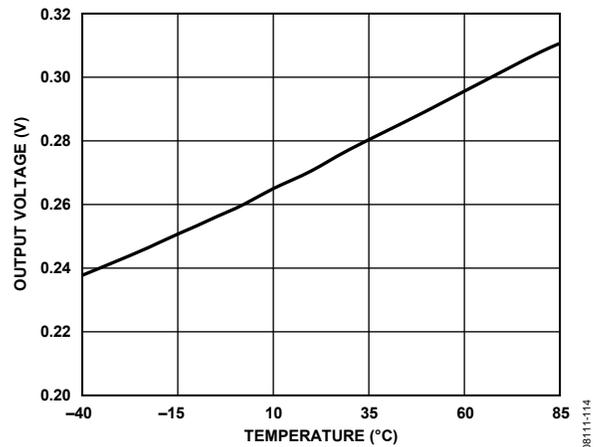
Figure 14. Receiver Output Low Voltage vs. Temperature
