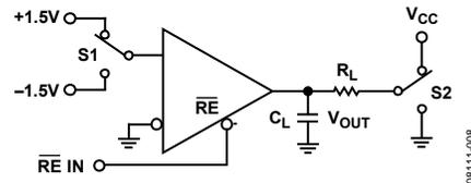
Figure 28. Receiver Enable/Disable
