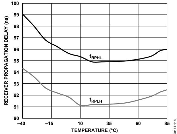
Figure 18. ADM2587E Receiver Propagation Delay vs. Temperature
