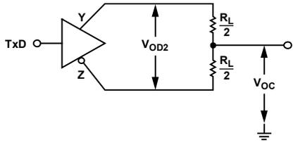
Figure 23. Driver Voltage Measurement
