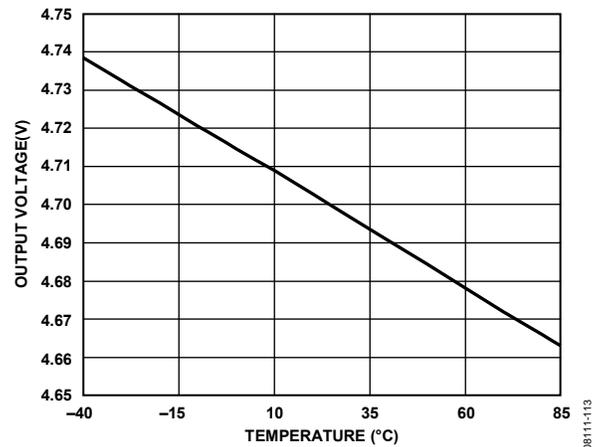
Figure 13. Receiver Output High Voltage vs. Temperature
