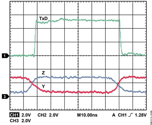
Figure 9. ADM2582E Driver Propagation Delay
