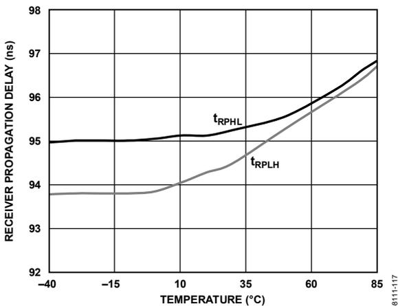
Figure 17. ADM2582E Receiver Propagation Delay vs. Temperature
