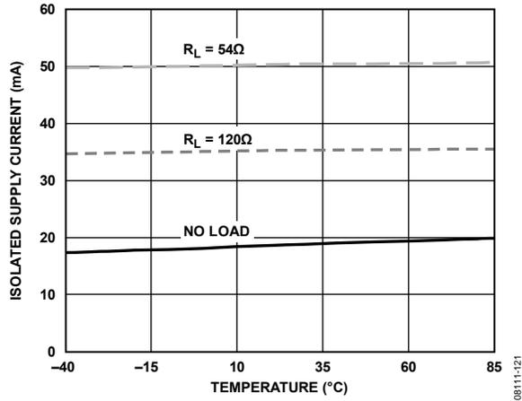
Figure 21. ADM2582E Isolated Supply Current vs. Temperature
