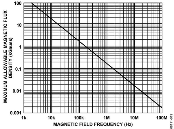
Figure 33. Maximum Allowable External Magnetic Flux Density
