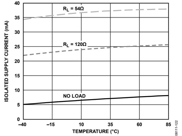
Figure 22. ADM2587E Isolated Supply Current vs. Temperature
