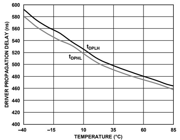
Figure 8. ADM2587E Differential Driver Propagation Delay vs. Temperature
