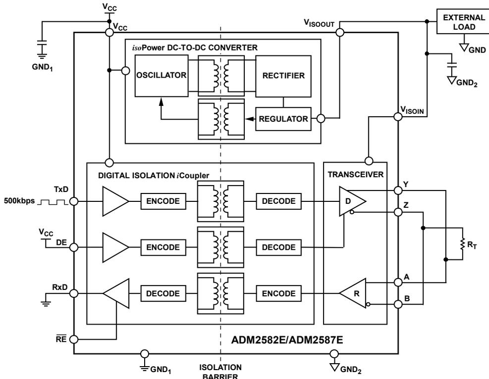
Figure 39. ADM2587E Typical Maximum External Current Measurements
