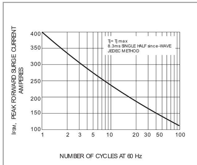
Fig.6 MAXIMUM NON-REPETITIVE PEAK FORWARD SURGE CURRENT UNIDIRECTIONAL
