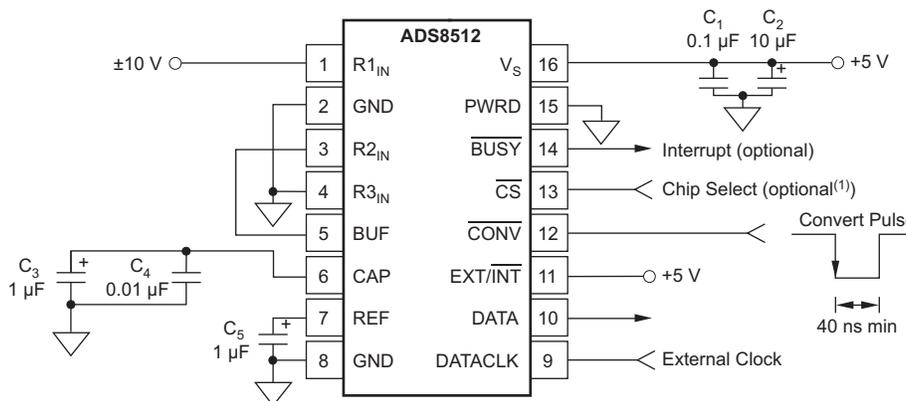
NOTE: (1) Tie  $\overline{\text{CS}}$  to GND if the outputs will always be active.
