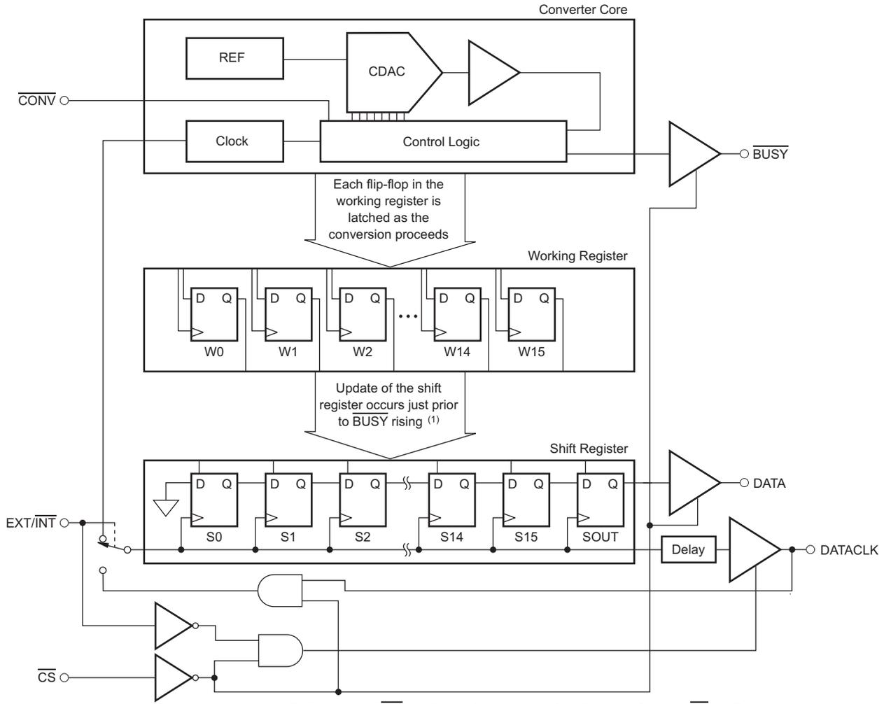
NOTE: (1) If EXT/INT is HIGH (external clock), DATACLK is HIGH, and CS is LOW during this time, the shift register will not be updated and the conversion result will be lost.
