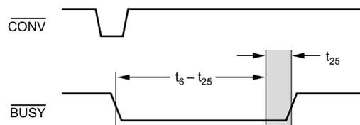
NOTE: Update of the internal shift register occurs in the shaded region. If EXT/INT is HIGH, then DATACLK must be LOW or CS must be HIGH during this time.
