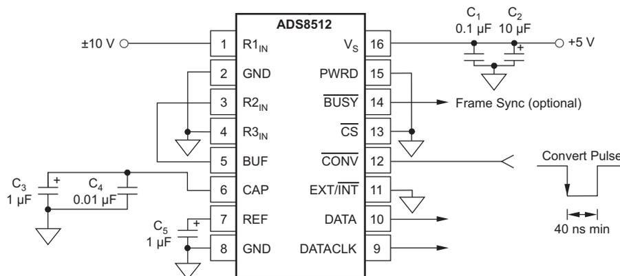
Figure 36. Basic Operating Circuit,  $\pm 10\text{-V}$  Input Range, Internal DATACLK
