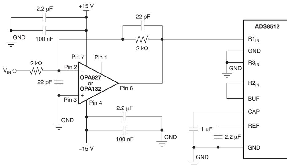
**Figure 46. Typical Driving Circuit ( $\pm 10$  V, No Trim)**
