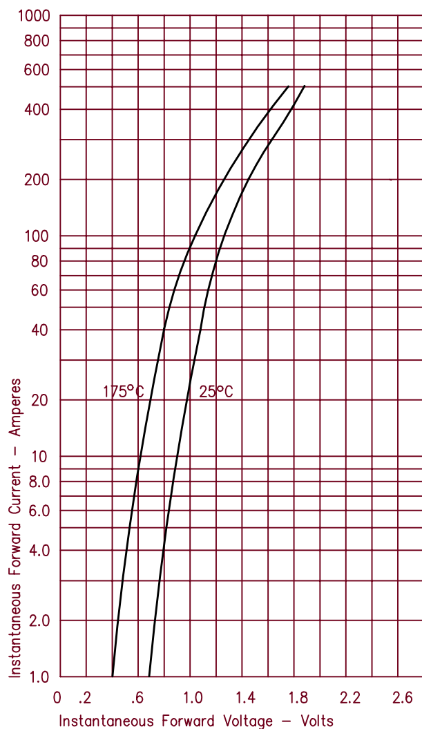
Figure 1 Typical Forward Characteristics
